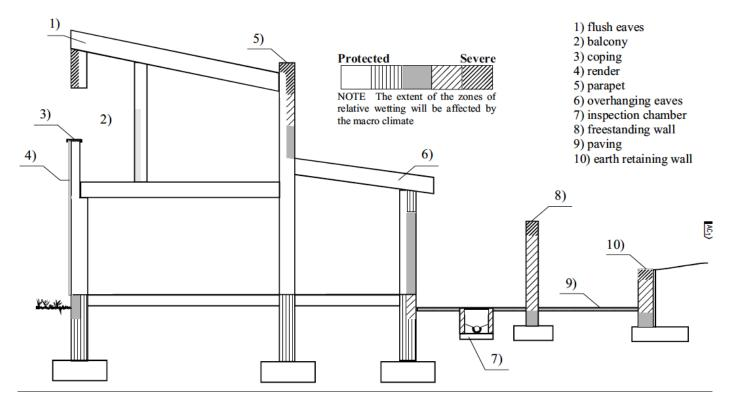
The following factors affect the resistance of brickwork walls to wind-driven rain. The order of the listing does not indicate relative importance. Each factor must also be considered in relation to other functions of the wall such as strength, durability, sound and thermal insulation:
