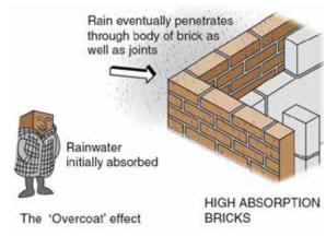
Although water absorption varies greatly between different bricks, this property has only a relatively small influence on the resistance of the finished wall to wind-driven rain. No difference is detectable between the rain resistance of brickwork built of the various forms of brick unit – solid, frogged or perforated. Also there is no evidence that rainwater collect in perforations during rainy periods, subsequently causing efflorescence or frost attack.
