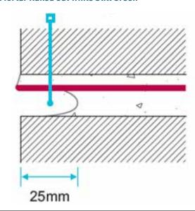
Flashing Wedged in Place and Pointed Up
